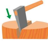
Wedae Made of wood or metal, this triangular tool can be used to push things apart.
