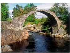
Arch Arch bridges are usually made of stones cut into exactly the right wedge shapes to form an arch.
