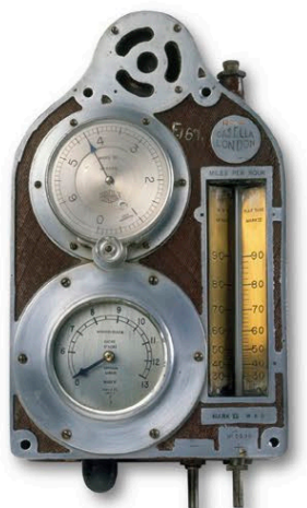
EARLY AIRCRAFT INSTRUMENT PANEL Showed aircraft's height and speed.
