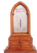
The electric telegraph, invented by William Cooke and Charles Wheatstone
