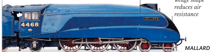
Body houses 5.5 m- (18 ft-) long, high-pressure boiler
